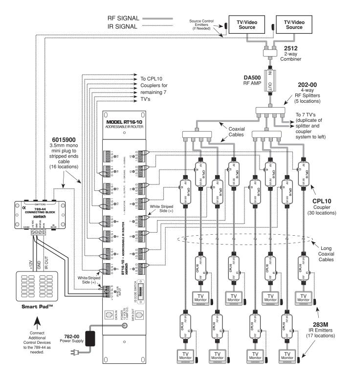
Fig. 7 Using the coaxial cables going to each TV to carry the IR Control Signals.
